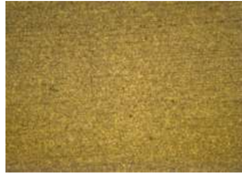
FIGURE 10. POROSITY TEST RESULT FOR NEW BATH
