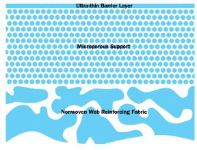
layer provides high water flux, unsurpassed salt and silica rejection, and excellent chemical resistance. The thick, microporous polysulfone support layer offers necessary porosity and strength properties and resists compaction under RO pressure conditions.
