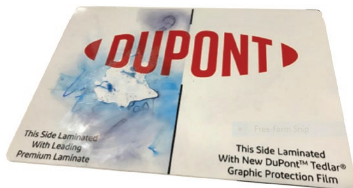
Figure 3: Extreme case demonstrating poor chemical compatibility of PVC and the exceptional cleanability and chemical resistance of Tedlar® PVF films.
