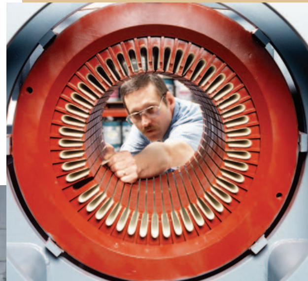
David Barnett inserting NOMEX® slot cells into a stator.
