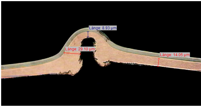
Poor copper throwing power
