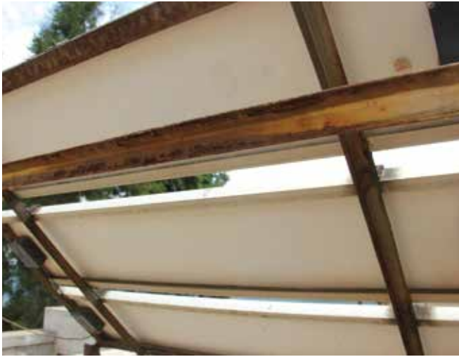
The frame and rack are rusty, but the DuPont™ Tedlar® PVF film-based backsheets are in excellent condition after 20 years of outdoor exposure. The PVF film on the back of the modules shows minimal yellowing, illustrating the excellent weatherability of the film
