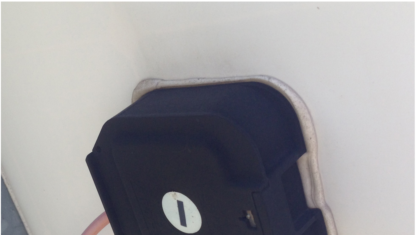
After 25 years of operation, the DuPont™ Tedlar® PVF film-based TPT backsheets on solar panels at the Mont-Soleil solar array remain in pristine condition.
