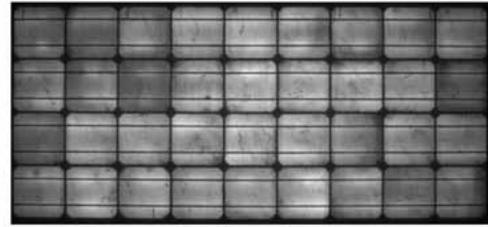
Figure 4 displays the condition of the module after 14 years of exposure to environmental conditions. The brighter areas indicate strong cell activity. There was no cracking observed and the power output is only 6% lower than the name plate power.
