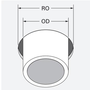
Use DuPont™ FlexWrap™ EZ only when penetration rough opening (RO) is not more than ½" larger than the outside diameter/ dimension (OD) of non-flanged product.
