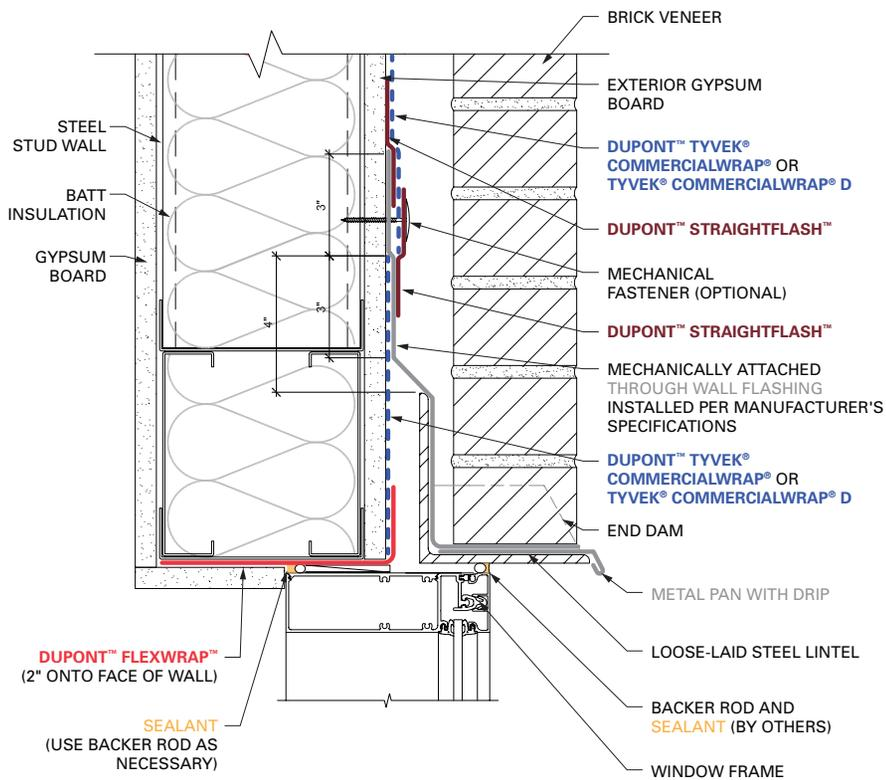
FLOATING LINTEL WITH METAL PAN AND MECHANICALLY ATTACHED THROUGH WALL FLASHING (SIDE VIEW)
