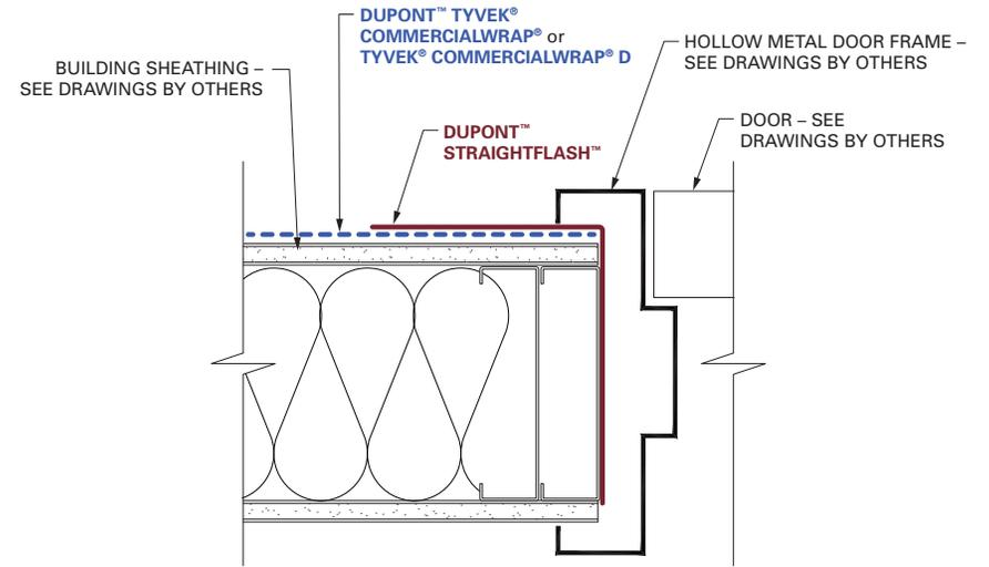
JAMB DETAIL (TOP VIEW) – HOLLOW METAL DOOR
