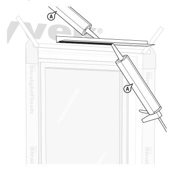
A. Place a bead of DuPont™ Sealant for Tyvek® Fluid Applied System, DuPont™ Residential Sealant, or recommended sealant, on the rear side of the vertical leg and a bead on the rear side of the bottom horizontal leg. Install the drip cap tight against the window head flange per the drip cap manufacturer's instructions.
