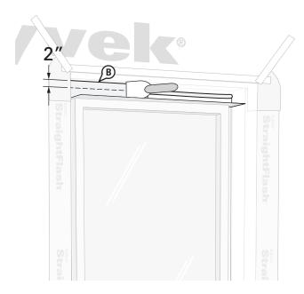
B. Apply a bead of DuPont™ Tyvek® Fluid Applied Flashing and Joint Compound+ along the top edge of the drip cap and trowel or brush to cover the vertical leg, extending 2" onto the recessed wall surface if possible.
