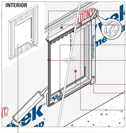
"1" cut WRB at rough opening with 45° cuts at window head extending min. 8" from corners. Flaps at jambs folded into the opening and secured.
